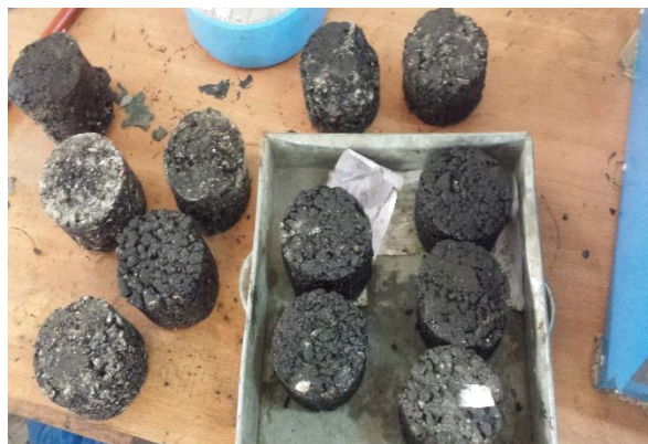
Figure: 3.1.3.1.6 Samples of Copper Slag Mix Asphalt
